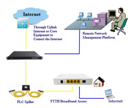
Figure: FD504G-E-R410 EPON ONU Application Diagram
